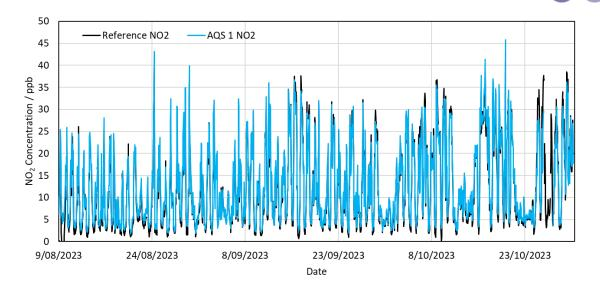
**Figure 7:** Hourly time series for AQS 1 and Thermo Scientific NO-NO<sub>2</sub>-NO<sub>x</sub> Analyzer from August 9<sup>th</sup> to October 30<sup>th</sup>, 2023, for the Calgary Inglewood station.
