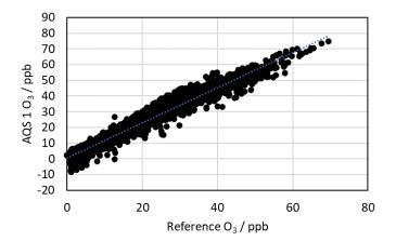
**Figure 5:** Scatter plot comparing hourly AQS 1 ozone module and Thermo Scientific Ozone Analyzer data for the Calgary Inglewood station from August 9<sup>th</sup> to October 30<sup>th</sup>, 2023.
