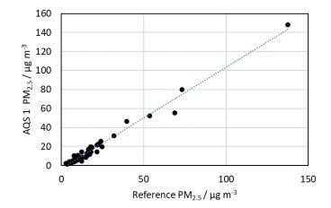
**Figure 11:** Scatter plot comparing the 24-hour AQS 1 PM<sub>2.5</sub> data and the Teledyne T640 PM<sub>2.5</sub> data from August 9<sup>th</sup> to October 30<sup>th</sup>, 2023, for the Calgary Inglewood reference station.
