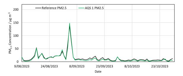
**Figure 10:** 24-hour time series data showing AQS 1 PM<sub>2.5</sub> data and the Teledyne T640 PM<sub>2.5</sub> data from August 9<sup>th</sup> to October 30<sup>th</sup>, 2023, for the Calgary Inglewood reference station.
