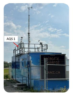
Figure 2: Calgary Inglewood reference station with AQS 1 installed on the roof.
