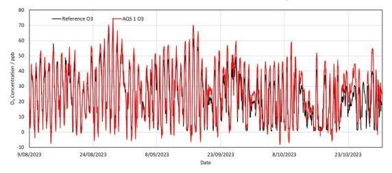
**Figure 4:** Hourly time series data for AQS 1 and Thermo Scientific Ozone Analyzer from August 9<sup>th</sup> to October 30<sup>th</sup>, 2023, for the Calgary Inglewood station.
