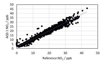
**Figure 8:** Scatter plot comparing hourly AQS 1 NO<sub>2</sub> module and Thermo Scientific NO-NO<sub>2</sub>-NO<sub>x</sub> Analyzer data for the Calgary Inglewood station from August  $9^{th}$  to October  $30^{th}$ , 2023.
