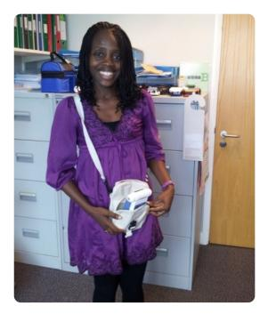
After consultation Dr Delgado-Saborit selected the Series 500 ENV fitted with a  $NO_2$  sensor head and optional temperature and relative humidity sensor. The ultraportable monitors have built-in data logging and lithium battery which would allow a full 8 hours operation in the field.
