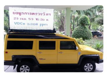
configured to continuously measure  $SO_2$ , CO,  $NO_2$ ,  $NO_X$ , VOC's and  $PM_{10}$ . Its lightweight and compact size also meant the AQM 65 was ideal for installation into a monitoring vehicle.
