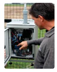
By using the Dust Sentry PC software Road Metals are able to extract data periodically without having to physically go to site. The modem also gives Aeroqual technicians the ability to connect with the instrument for running system checks and remote diagnosis.
